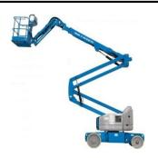
This lift has at least 2 hinged sections which are used to increase mobility.
